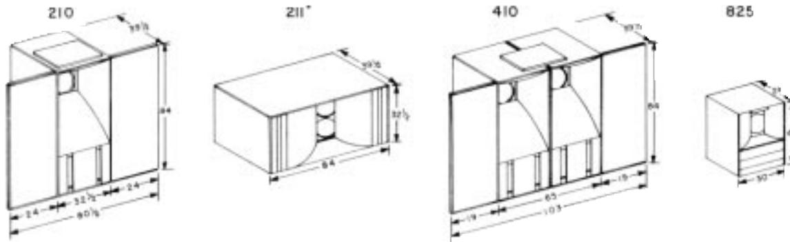
FIGURE 1: Dimensional drawings of Altec Low Frequency Horns.
